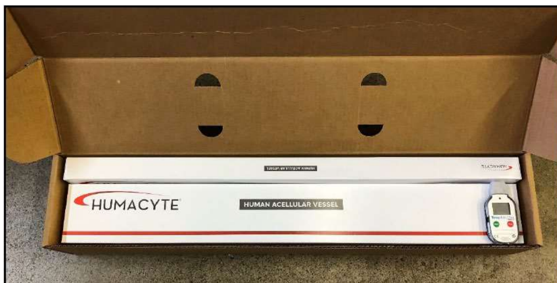
Figure 23 – Payload Box with Max Load (b) (4) units) and Temperature Logger (Reproduced from Page 11 of A50 34L9-HUB-RF-96 Physical Testing Report v1 in Submission 0001)
